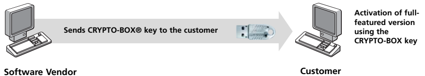
Figure 1.4 A typical example of a smart ESD strategy - implemented with the CRYPTO-BOX key
